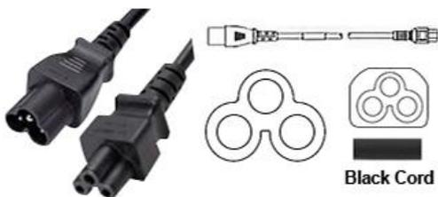
**IEC C5/C6 connectors** are a very common type of personal/home power connector. They are rated for 250V/2.5A and include an earth (safety) ground wire. They are commonly called a clover leaf or a Mickey Mouse (after the Disney cartoon character) connector due to their cross-sectional shape. C5/C6 connectors are commonly used on laptop power supplies.
