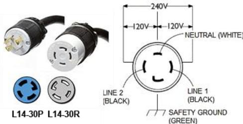
One of the advantages of NEMA connectors is the wide variety of power distribution systems for which it can provide a separable power connection. For example, a NEMA L14-30 connector is capable of connecting loads to two-pole, four-wire, 240/120 VAC power systems up to 30A. This type of multi-voltage connector simplifies installation by reducing the need and cost of hard-wiring multiple connections, while the locking feature aids in connection security.
