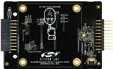
Biometric Sensor Expansion Card for EFM32™ Wonder Gecko Starter Kit
