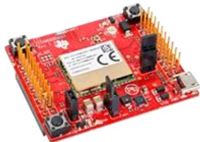
*CC3100MOD SimpleLink™ Wi-Fi® Network Processor Module BoosterPack*
