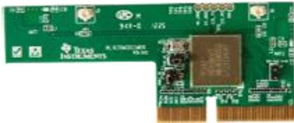
WiLink™ 8 Module 2.4 GHz Wi-Fi® + Bluetooth® COM8 Evaluation Module
