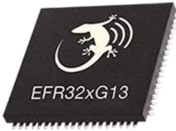
*EFR32BG13 Bluetooth SoC Microcontroller QFN48*
