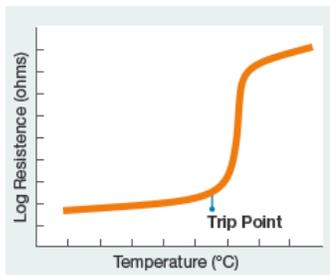
Figure 5: Response of PTC Resistance to Temperature
