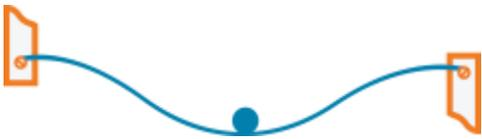
Figure 3: The ball on wire fuse invented by AC Cockburn
