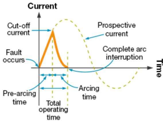
Figure 4: Fuse Operation During Fault Condition
