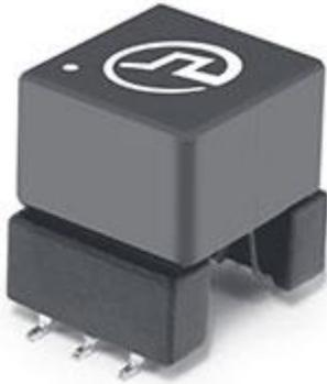
*Figure 15: Pulse Electronics PH9185 is a high isolation power supply transformer driver. It's intended to operate in a fixed duty cycle Push Pull topology. A typical implementation would be an isolated RS-485/RS-232 power supply driver circuit.*
