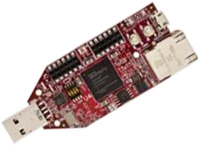
*Avnet Spartan-6 FPGA LX9 Microboard*
