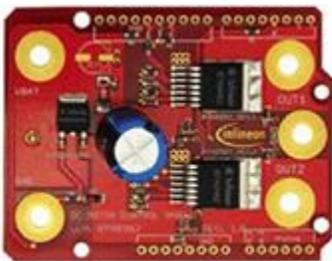
**Motor Control Shield with BTN8982TA for Arduino**
