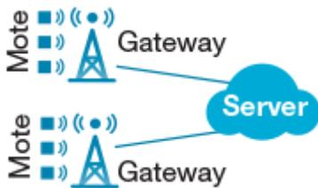
Figure 6: Mote to Gateway is a One Hop Transmission
