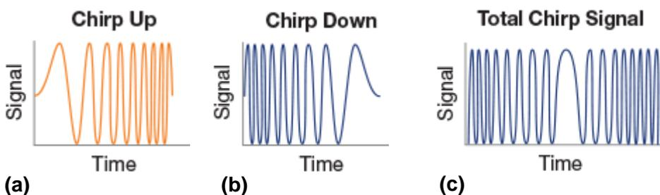
Figure 7: Chirp modulation uses sinusoidal waveforms whose instantaneous frequency increases (a) or decreases (b) over time. LoRaWAN transmissions work by chirping, that is, separating the chirps in various places relative to time and frequency to encode information (c).
