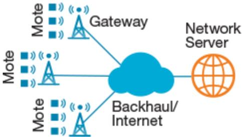
Figure 5. A typical LoRaWAN network architecture (Source: *Experimental Performance Evaluation of LoRaWAN: A Case Study in Bangkok/IEEE*).
