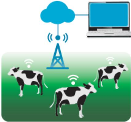
Figure 3: LoRa Livestock Monitoring System
