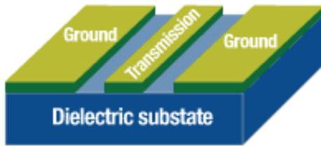
Figure 8: Coplanar Waveguide
