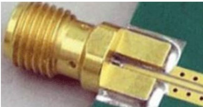
Figure 15: Clean Flux and Residues
