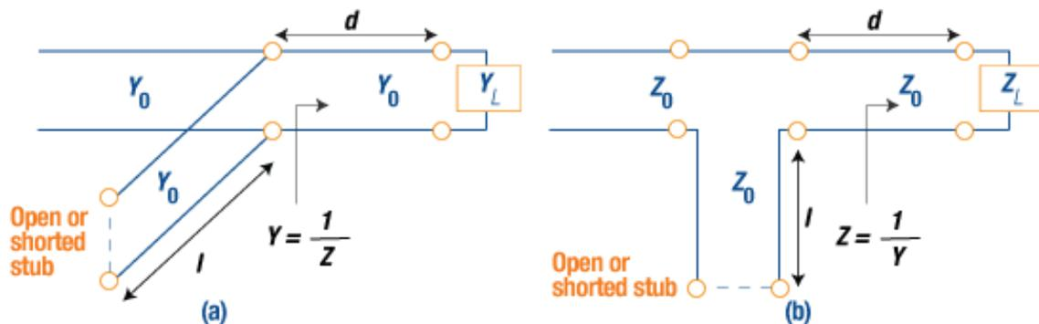
Figure 10: Single Stub Matching: Parallel (a); Series (b)
