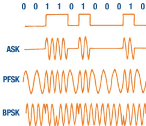
Figure 4: Output of ASK/FSK/PSK Modulation Schemes
