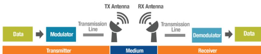
Figure 1: A simple RF communication system block diagram
