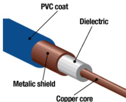
Figure 5: Coaxial Cable
