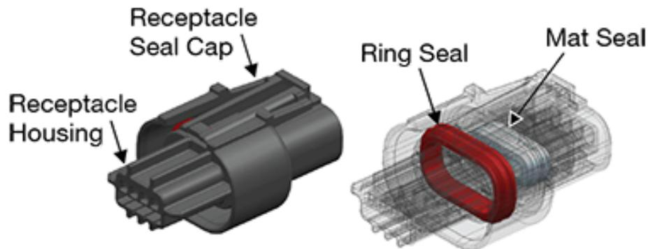
Figure 3: Connector Assembly
