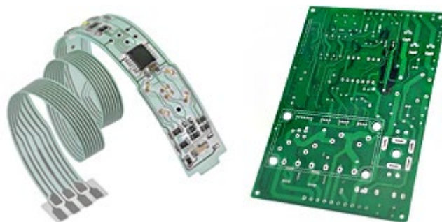
Figure 1: Silver Flexible Printed Circuit (FPC) Board Technology (Left) from Molex and Rigid Printed Circuit Board
