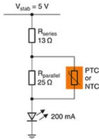
Figure 2: Temperature-compensated LED driver without an IC
