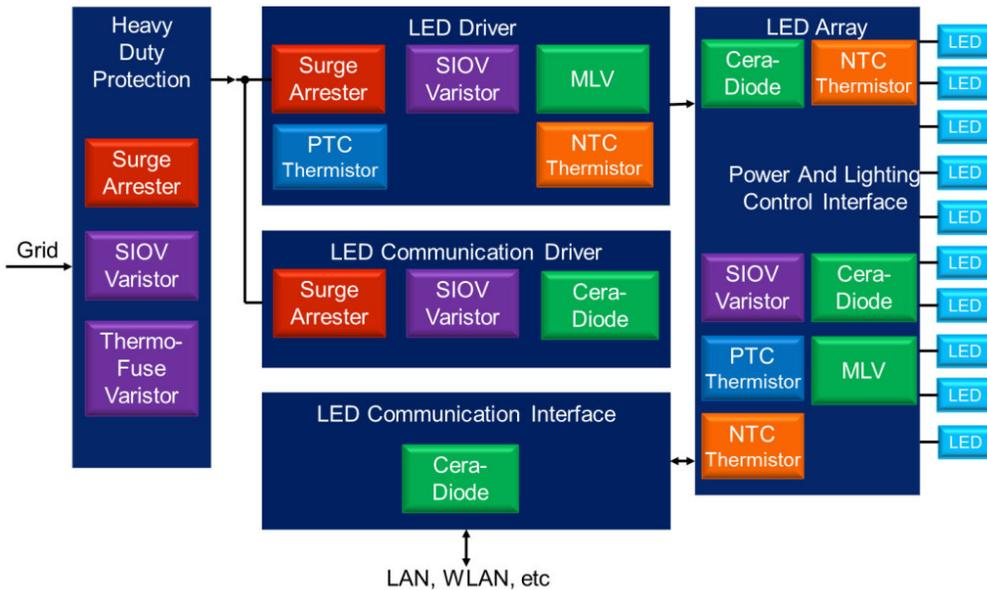
Figure 1: Overview of the subsystems and their suitable protection devices.
