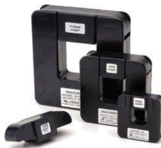
Figure 5. Split core CTs typically have a hinge or removable section for installation around a line without physical disassembly, though the power should still be disconnected. (Image courtesy of Magnelab)
