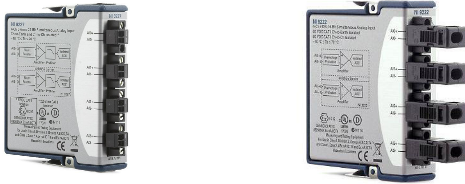
Figure 1. The NI 9229, NI 9239, NI 9227, and NI 9238 have a two terminal connector (left) for each measurement channel. Shields are available (right), and recommended, for strain relief and operator keep-outs from connections to active circuits.
